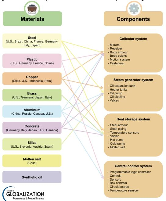
Figure 4-3: CSP Components and Materials with Top Producing Countries
