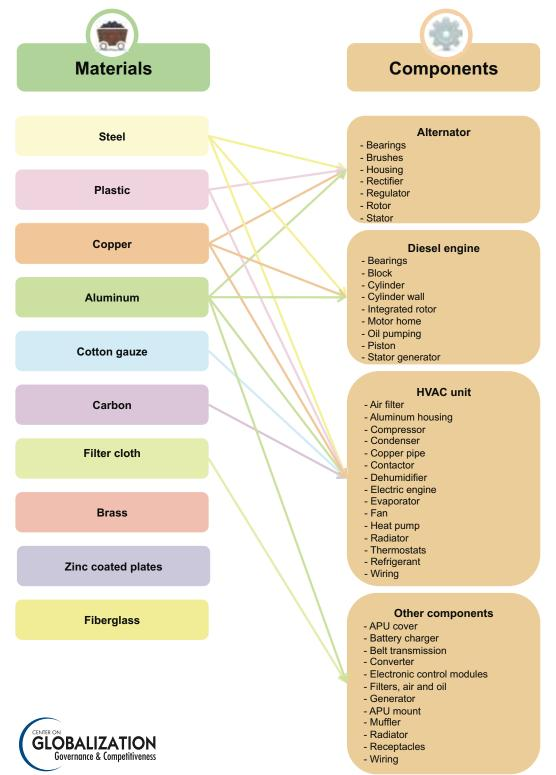
Figure 3-3. Auxiliary Power Unit Materials and Corresponding Components
