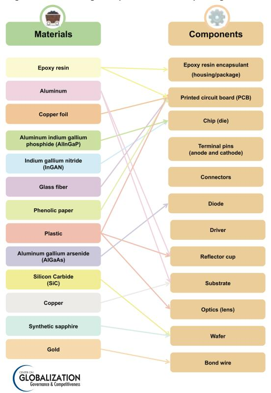
Figure 1-4. LED Package Components and Corresponding Materials\*
