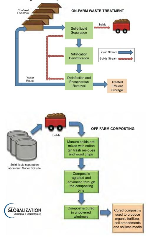
Figure 5-2. Super Soil Waste Treatment Process
